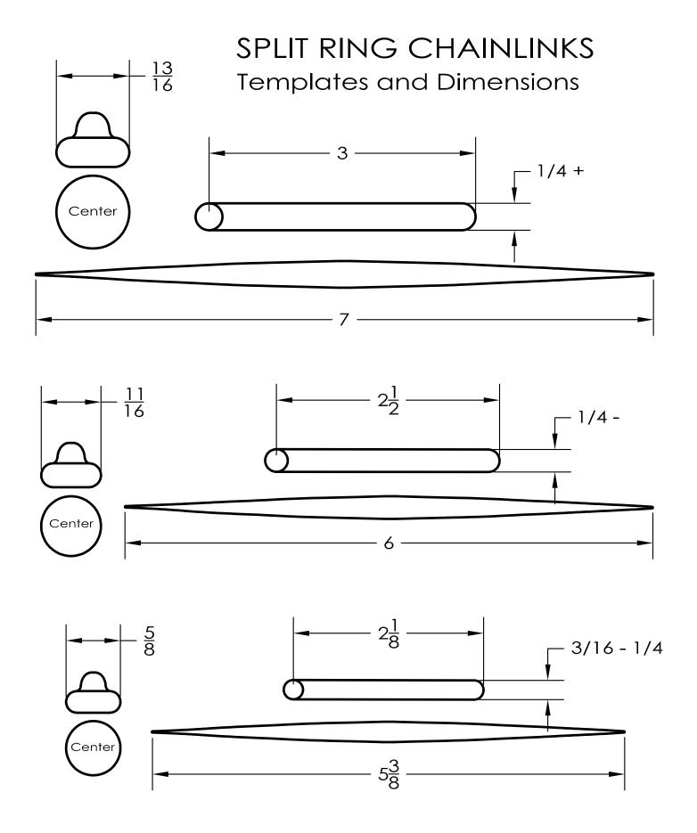
Make centers by squashing a ball of clay to the size shown and adding a small handle. Bake according to the manufacturer's instructions.
